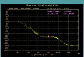
Phase Noise at 4 GHz and 8 GHz. Phase noise of better than -100dBc/Hz at a 10kHz offset make the 20309 the ideal L.O. for radar/FW testing
