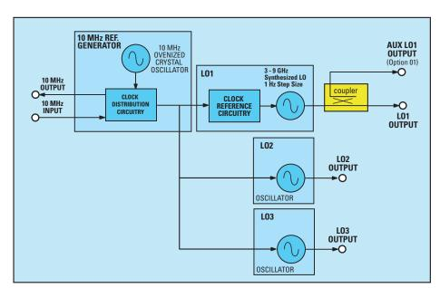
Simplified Block diagram of the Phase Matrix Model 20309.
